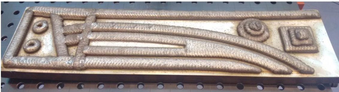
Figure 24 : Lortek plot 3 demonstrator in Stainless Steel
