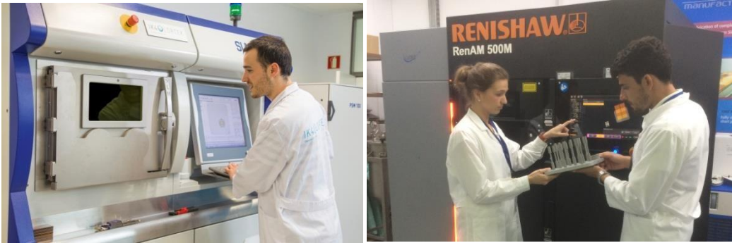
Figure 32: Powder Bed Fusion machines used in order to manufacture the demonstrators
