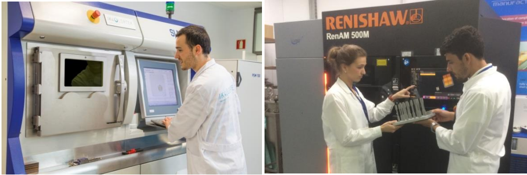
Figure 2. Powder Bed Fusion machines used in order to manufacture the demonstrators.
